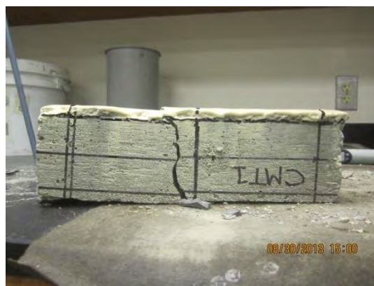
Figure C-22. Specimen CMT1#1 at Failure.
