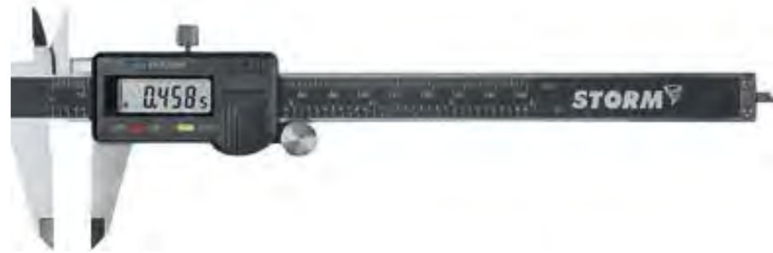
Figure 4-7. Digital Caliper Used for Measuring Specimen Dimensions.
