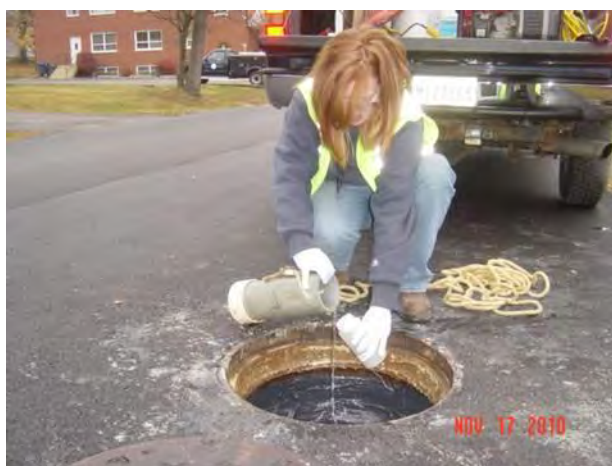
Figure 6-19. Village Employee Collecting Wastewater Sample to Analyze for Ammonia Concentration.
