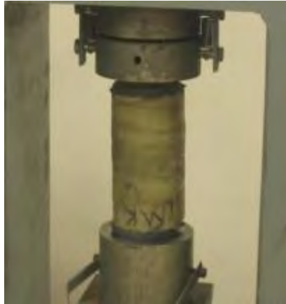
Figure C-33. Lined Cylinder CIP-C Specimen Mounted on the Admet 500 Kip Compression Test Machine.
