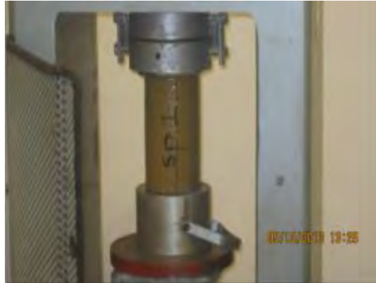
Figure C-39. Lined Cylinder CIP-C Specimen Mounted on the Admet 500 Kip Compression Test Machine.
