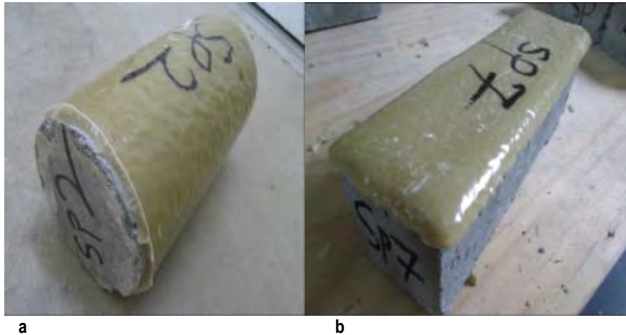
Figure 4-5. Concrete Cylinder (a) and Beam (b) Samples Lined with High-Build Polyurethane.
