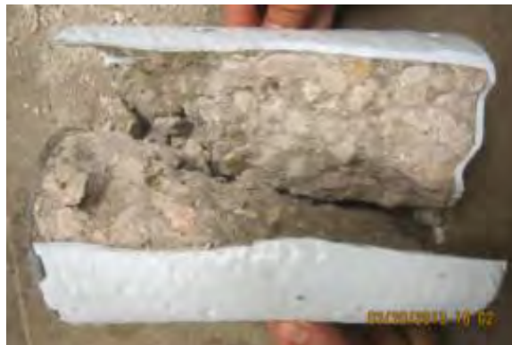
Figure C-32. Specimen EPX1-C#5 Failure Pattern.
