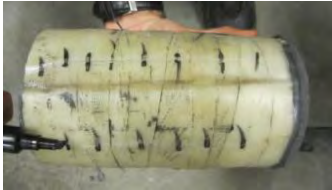
Figure C-35. Specimen CIP-C#2 at Failure, Note the Circumferential Cracking.
