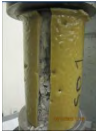
Figure C-40. PU-C#1 Failed with a One-Inch (25 mm) Wide Fracture
