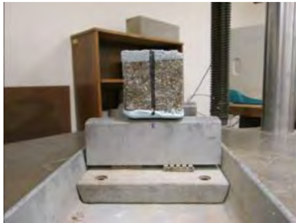
Figure C-4. Cross-Section of EPX1-F#3, Note the Variation in Lining Thickness Across the Specimen.
