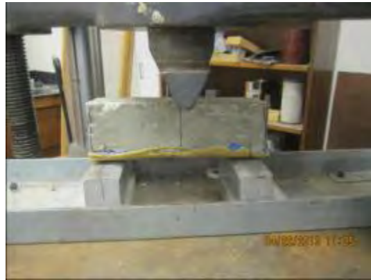
Figure C-15. Polyurethane (PU) Beam Specimen Mounted on the Baldwin 60 KIP for the Flexure Test.
