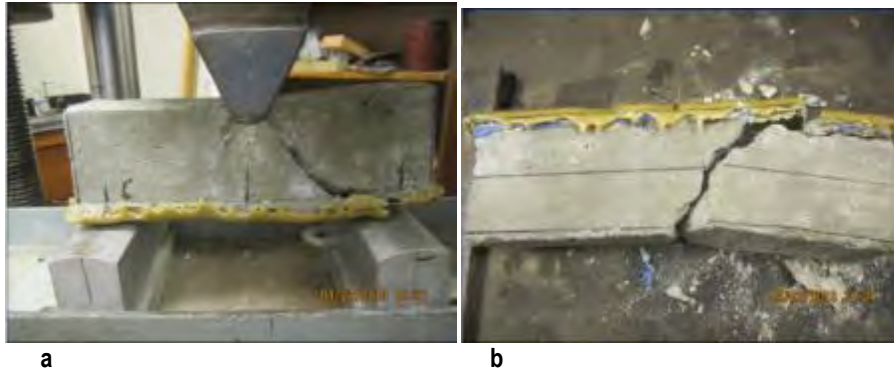
Figure C-19. Specimen PU-F#6 at Failure (a) with a Thin Section Separating Near the Support (b).
