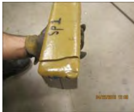
Figure C-16. Specimen PU-F#1 Liner Failure at the Support.
