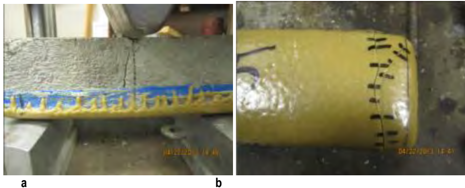
Figure C-18. Fracture in the Concrete Substrate (a) and PU-F#5 Liner Failure at the Support (b).
