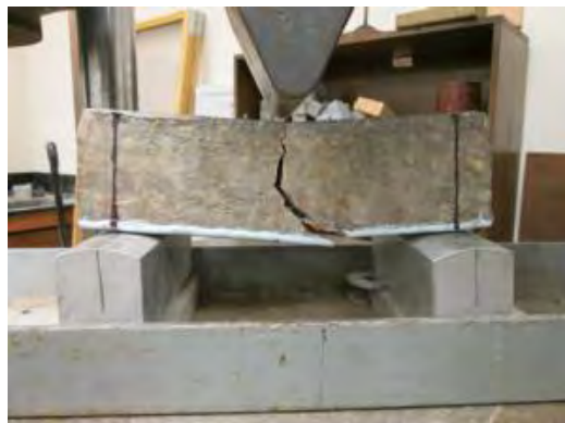
Figure C-5. Specimen EPX1-F#3 at Failure, Note the Inclination in the Failure Plane.
