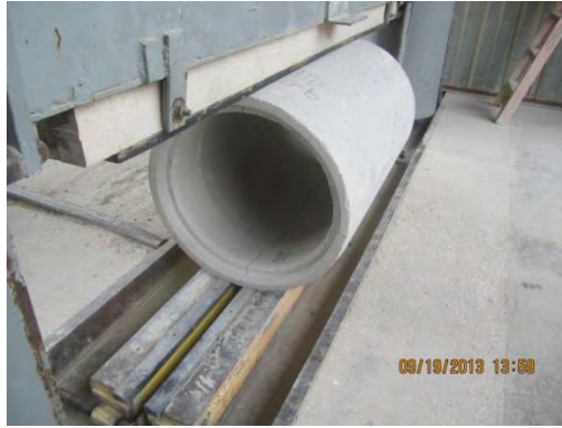
Figure 4-18. Pipe Crushing Test Setup per ASTM C497.
