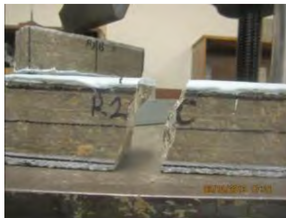
Figure C-3. Failure of Specimen EPX1-F#2.
