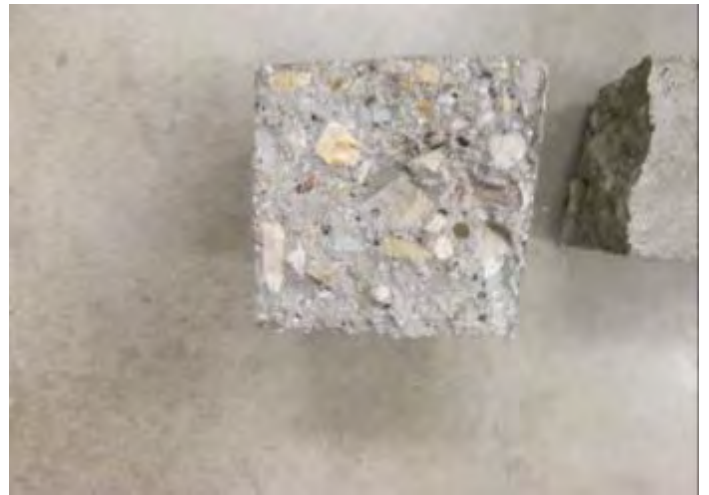
Figure 4-12. Unlined (Control) Beam After Testing.
