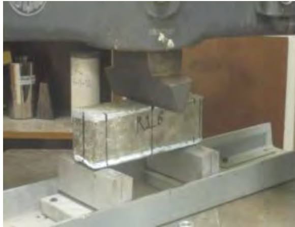
Figure C-1. EPX1-F#1 Mounted on the Baldwin 60 KIP for the Flexure Test.
