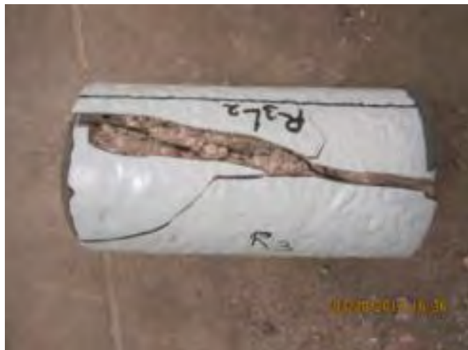
Figure C-30. Specimen EPX1-C#3 Failure Pattern.
