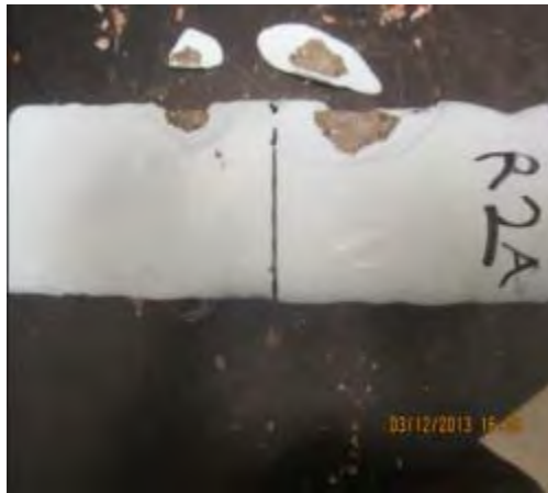
Figure C-2. Liner Pieces Chipped off EPX1-F#2 During Shipping.
