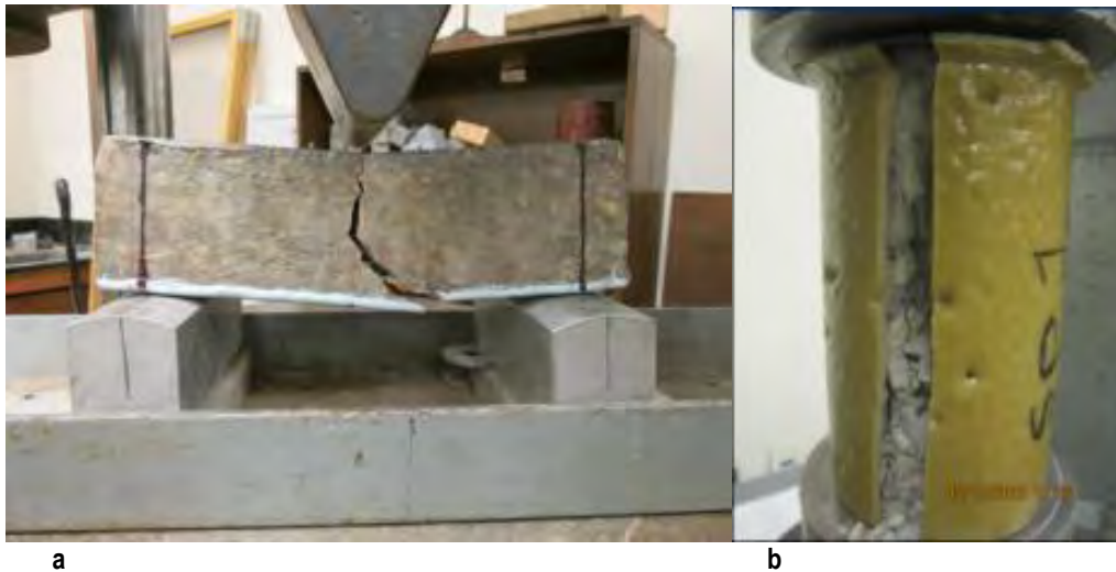
Figure 4-13. Beam (a) and Cylindrical (b) Specimens at Failure While Loaded for Flexural and Compressive Strength, Respectively.
