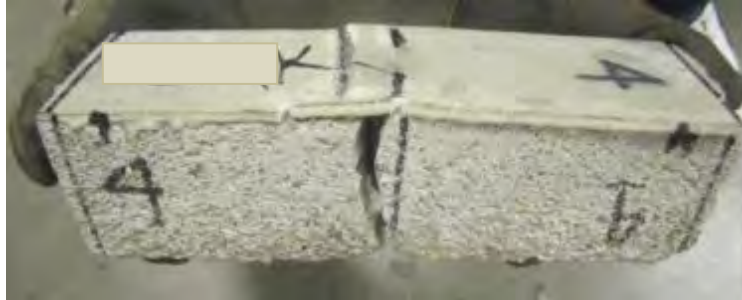
Figure C-13. Specimen CIP-F#4 at Failure.
