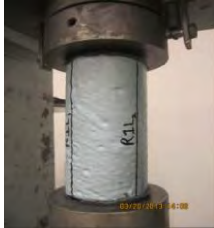
Figure C-27. Lined Cylinder Specimen Mounted on the Admet 500 Kip Compression Test Machine.
