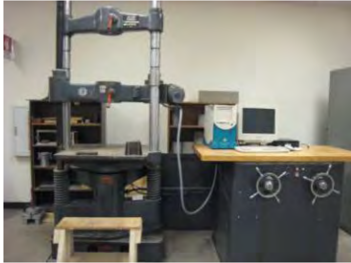
Figure 4-2. Baldwin 60 KIP Flexural Strength Testing Machine.
