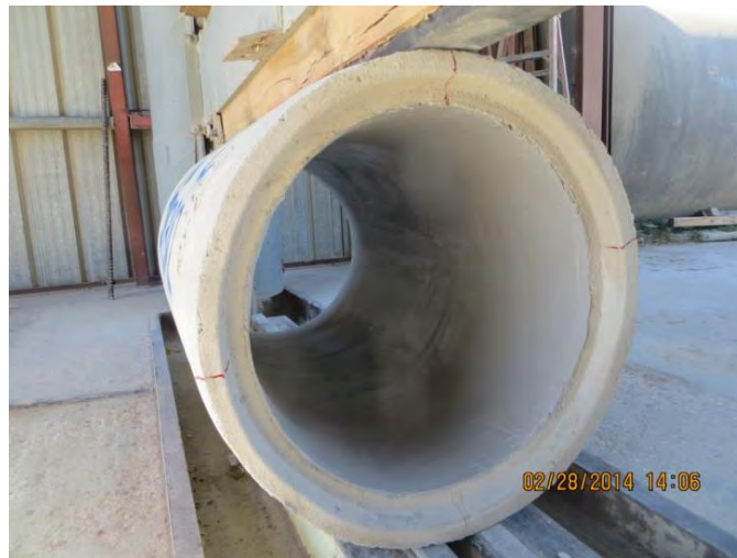
Figure 4-22. Example of Failure by Cracking in the Concrete Substrate Only.
