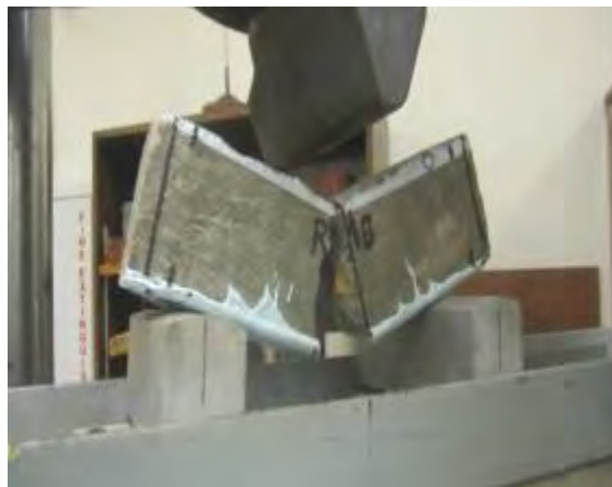
Figure C-7. Specimen EPX1-F#4 at Failure.
