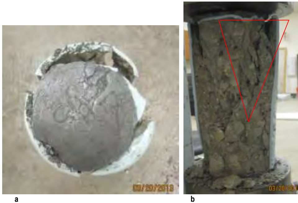
Figure C-31. Specimen EPX1-C#4 at Failure (a) with a Cone-Shaped Fracture Pattern in the Concrete Core (b).
