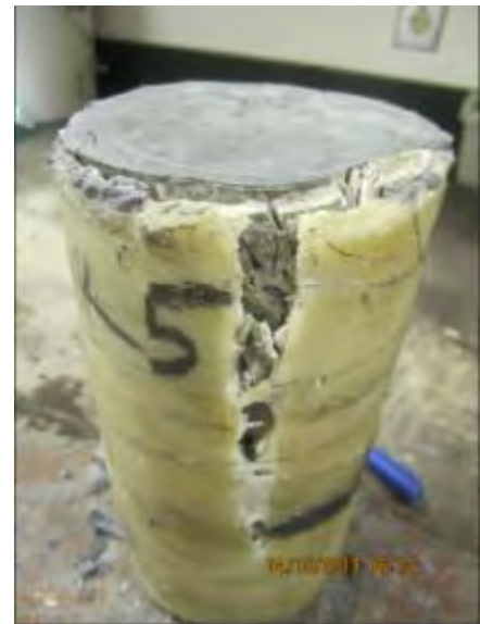
Figure C-38. Specimen CIP-C#5 Failure Pattern, Note the Vertical Splitting.
