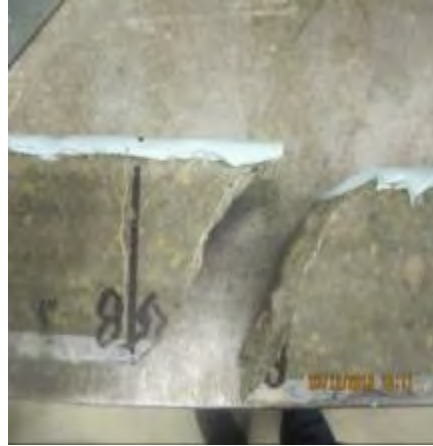
Figure C-8. Failure Pattern of EPX1-F#5.
