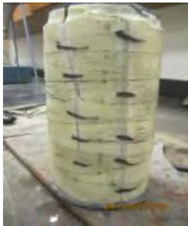
Figure C-34. Specimen CIP-C#1 at Failure, Note the Liner Did Not Separate From the Concrete Substrate.
