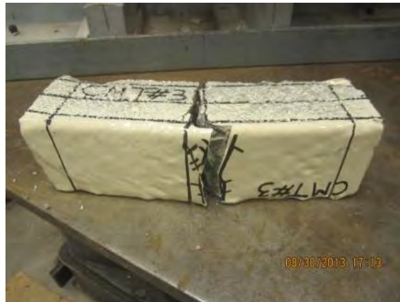
Figure C-24. CMP-F#3 After Tested to Failure, Note the Crack (Fracture) Line.
