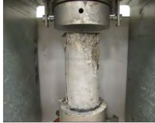
Figure 4-10. Unlined (Control) Cylinder After Testing.
