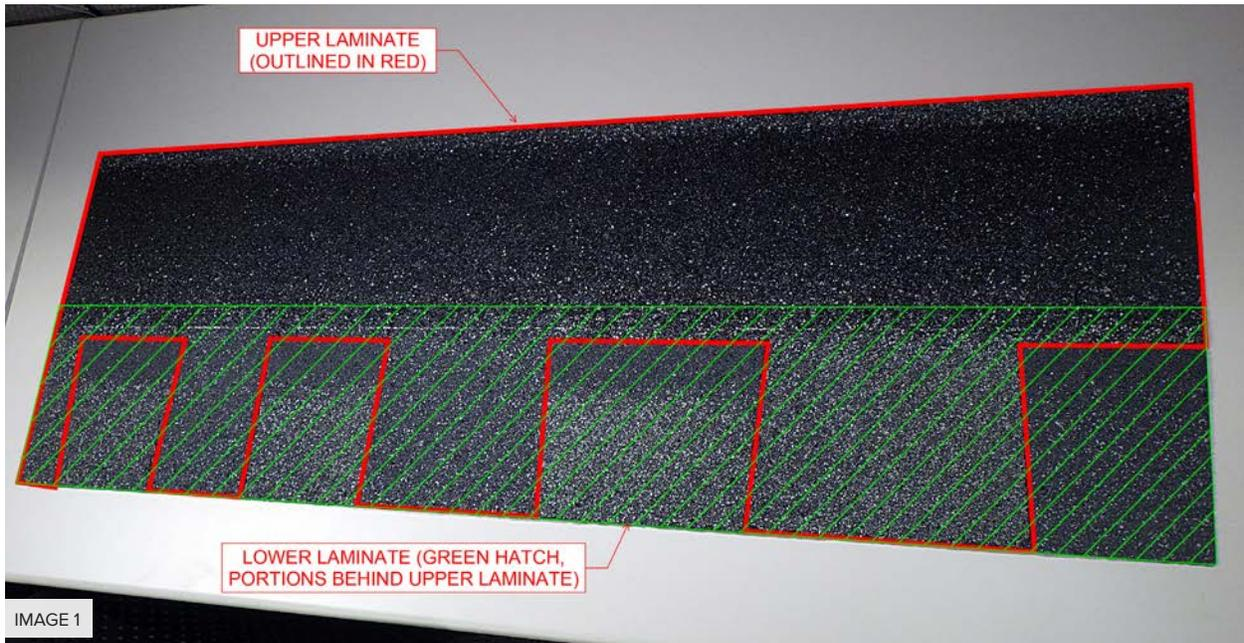
The upper laminate, or sawtooth section, typically extends the full shingle height (commonly ranging from 12 inches to 13.25 inches), with cutouts in the lower, exposed portion of the shingle to create the “sawtooth” or “dragon tooth” appearance (see Image 1).
