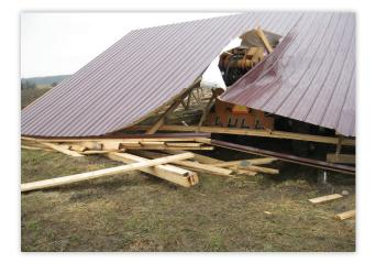
a compression brace to each adjacent wall stud significantly reduces its capacity to the point where the long and flimsy brace easily kicks out of plane and buckles in compression as was observed. When the compression braces suddenly fail, the entire wind load must be resisted by the tension braces. In this case, the entire wind load that was transferred to the tension braces resulted in failure of the connection between the tension braces and the wall studs.
